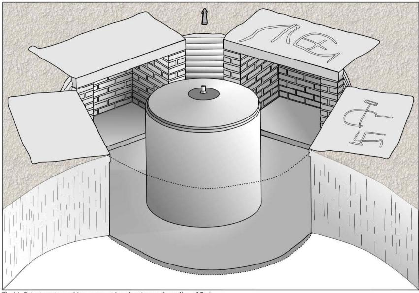
Fig 14 Spigot mortar position - perspective view (arrow shows line of fire)
