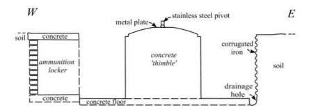
Fig 13 Spigot mortar - section
